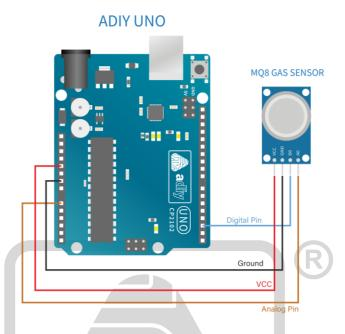
Note: You should always allow some time for the sensor to pre-heat before reading the output data.
