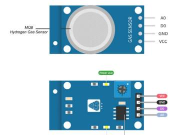
VCC: Voltage input for module
